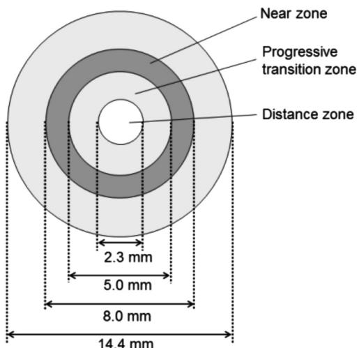
**Figure 1 Optical design of the refractive multifocal contact lens (ROHTO i.Q 14 Bifocal D-type)** The refractive multifocal CL used in the current study consists of three zones, with distance, progressive transition, and near zones in order from the central to the peripheral zones, respectively. Additional power for near vision is +2.50 diopter.
