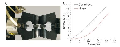
**Figure 7 Illustration of biomechanical test** A: Biomechanical test of scleral strips on an Instron 5565 universal testing machine; B: Stress-strain curve of tensile test. Two lines were chosen from one subject in this study. Ultimate stress of sclera in the LI eyes was lower than that in contralateral eyes (13.53 vs 18.65 MPa, *P*=0.021). Young's modulus was lower in the LI eyes than that in control eyes (0.4740 vs 0.8145 MPa, *P*=0.043). LI: Lens-induced.
