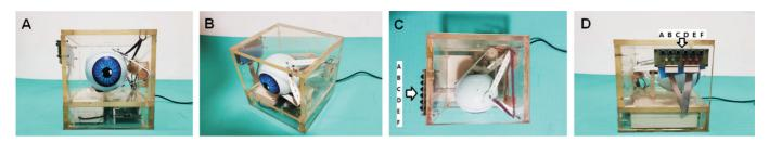
Figure 3 Photo of 3D electric ophthalmotrope A: Positive view; B: The lateral view; C: The above view; D: Control buttons.
