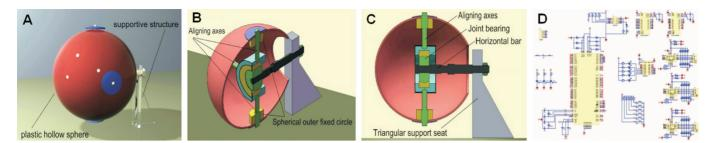
**Figure 1 External and internal views of the shell and circuit diagram** A: Spherical shell containing a plastic hollow sphere and supportive structure; B: Internal structure including a joint bearing, four aligning axes, horizontal bar and a triangular support seat; C: Planar graph of internal structure view; D: Circuit diagram of electrical control system.
