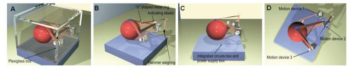
**Figure 2 Design drawing of 3D electric ophthalmotrope** A: The lateral view with exterior frame; B: Lateral view without the frame, showing that an elastic band starts from above the spherical shell through the "U" shaped metal ring witch simulated tackle, and further extends to the left rear. A lead hammer is used to maintain its extension. C: An integrated circuits box and power supply are located on the bottom of the sphere model; D: The location of the three-motion device.
