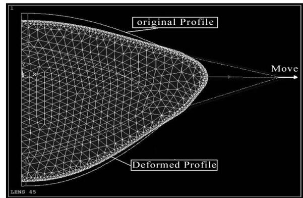
Figure 4 Lens deformation with pull displacement=0.1mm
