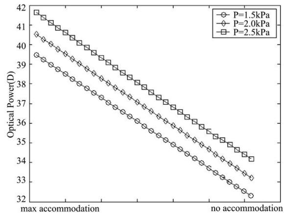
**Figure 8 Lens variation with different displacements with  $P=1.5, 2.0, 2.5\text{kPa}$  respectively**
