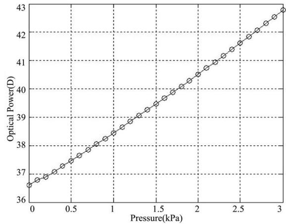
**Figure 7 Variation of the optical power with pressure**
