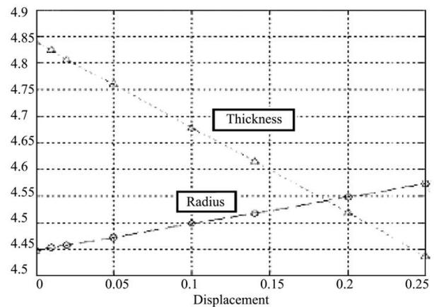
Figure 5 Lens thickness and radius variation with displacement
