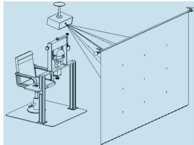
**Figure 1** Schematic diagram of the device for applying the computerized diplopia test.
