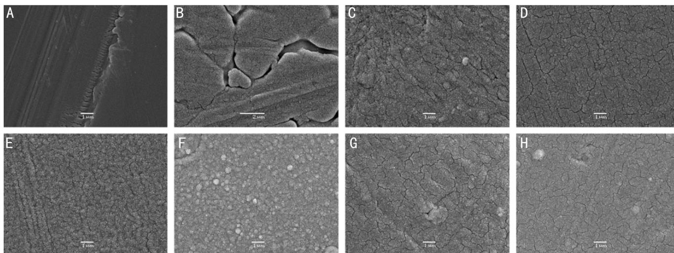
**Figure 3 Scanning electron microscopy of the selected materials** All images were taken at 10 000 magnifications. Steel was the only material with grooves of a size similar to the bacterial diameter. A: Glass; B: Steel; C: Teflon; D: Polymethylmethacrylate; E: Orbital implant silicone; F: Commercial silicone; G: High density porous polyethylene; H: Semi-smooth polyethylene.
