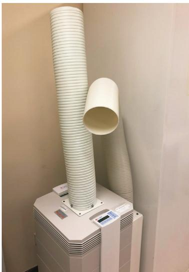
Figure 6 Portable HEPA filter unit.
