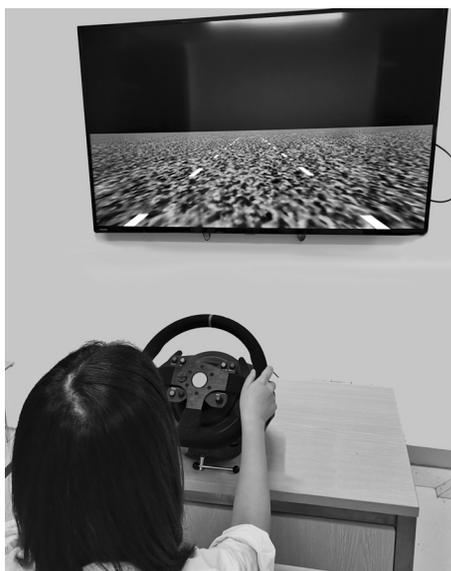
**Figure 3** Set up of the driving simulation test with participant being under examination.
