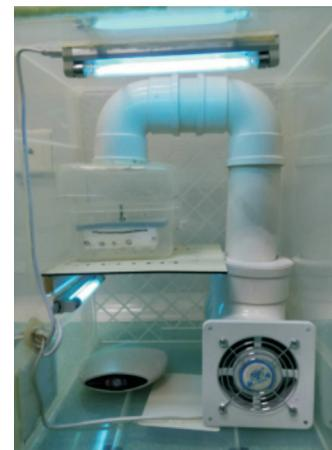
**Figure 2** The internal structure of dehydrater.
