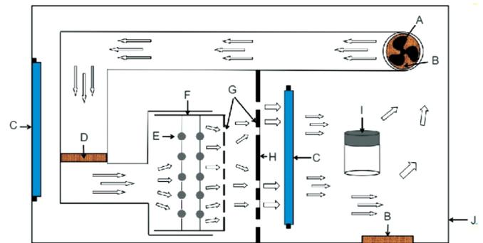
**Figure 1** The schematic diagram of the dehydrater A: Circulating fan; B: Dustproof filter screen; C: Ultraviolet lamp tube; D: Dustproof filter screen; E: Positioning hole; F: Dehydrating box; G: Air vents; H: Fixed platform surface; I: Regenerative humidifier; J: Sealed working box.
