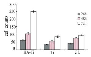
Figure 3 Cell counts on test materials hydroxyapatite modified titanium (HA-Ti), pure titanium (Ti), glass (GL) at 24, 48, and 72 hours
