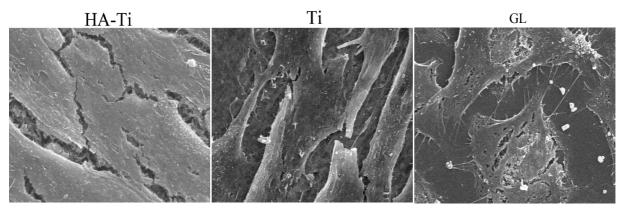
Figure 5 Scanning electron microscopy showing cell spreading area on hydroxyapatite modified titanium(HA-Ti), titanium(Ti), and glass(GL)
