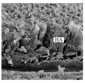
Figure 1 The thickness of the HA was seen about  $20\mu m$  after the deposition on the new-cut side face (NC). Arrows indicate the interface of the surface HA/.Ti substrate
