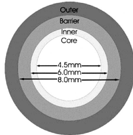
Figure 6 Cross section of the lens.
