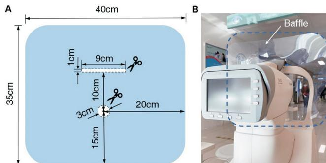
**Figure 3 Production and installation of the baffle** A: Select a plate made of transparent plastic, cut according to the dotted line and grind the four corners to be blunt; B: Install and fix the baffle at the jet port (the air jet of the NCT passes through the round hole of the baffle), between the display screen and the head rest of the patient (dotted blue outline).
