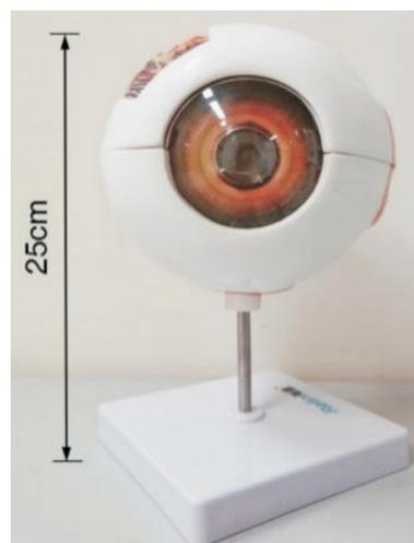
**Figure 1 A frontal diagram of the model eye** The height of the model eye is 25.0 cm, the eyeball diameter is 13.5 cm, the iris diameter is 6.0 cm and the pupil diameter is 2.5 cm.
