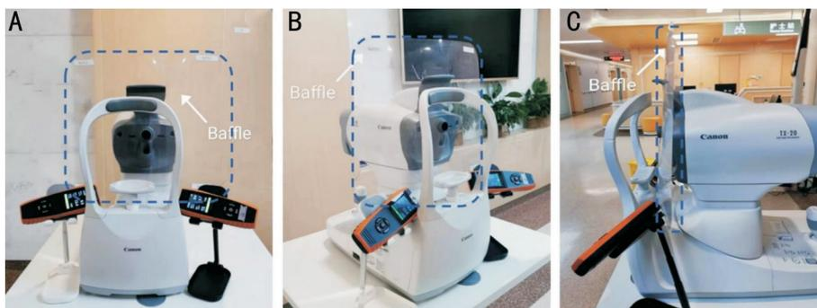
**Figure 2 Location of two air quality detectors** A: Anterior; B: Left lateral; C: Right lateral. During the trial, both air quality detectors were fixed at the groove between the jet port and the chin rest. When the baffle was installed (dotted blue outline), the detectors were fixed in the same position in front of the baffle, leaning towards the side of patient.
