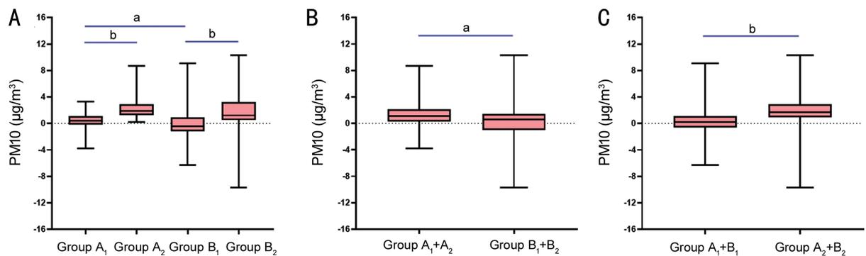
**Figure 6 Comparison of effects of baffle and IOP on per capita PM<sub>10</sub>** A: Comparison of four groups; B: Group A<sub>1</sub>+A<sub>2</sub> versus Group B<sub>1</sub>+B<sub>2</sub>; C: Group A<sub>1</sub>+B<sub>1</sub> versus Group A<sub>2</sub>+B<sub>2</sub>. Boxes represent interquartile ranges. Whiskers represent the lowest or highest data point still within a 1.5 multiple of the interquartile range. <sup>a</sup>*P*<0.01, <sup>b</sup>*P*<0.001.
