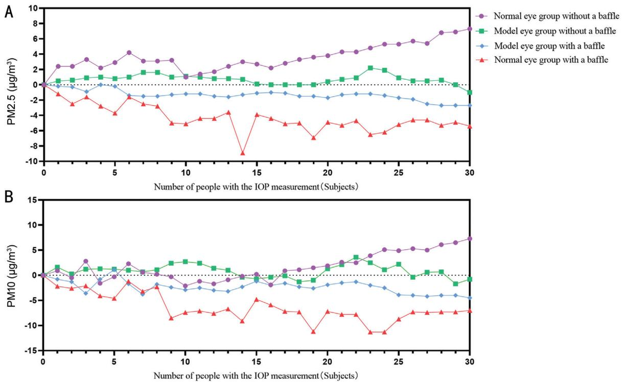
**Figure 4 Comparison of effect of baffle on aerosols accumulation A: PM<sub>2.5</sub>; B: PM<sub>10</sub>.** The 0 value of each y-axis indicates the initial aerosol density before the IOP measurement. The negative value of each y-axis indicates that the aerosol density after IOP measurement is lower than the initial density. The positive value of each y-axis indicates that aerosol density after IOP measurement is higher than the initial density.
