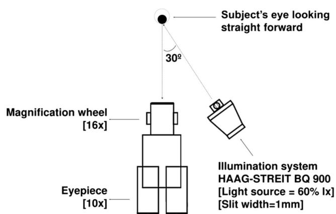
**Figure 1** Schematic diagram of the anterior slit photograph imaging process.
