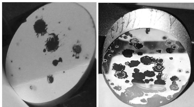
**Figure 1 Degraded mirrors for reflection of IR illumination (eye tracking).**
