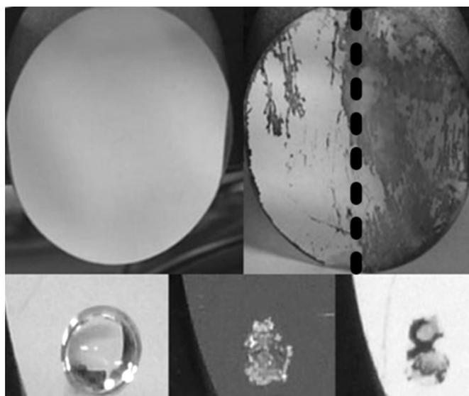
**Figure 2 IR mirror degradation upon UV-C radiation** From left to right, the new and the washed out after degradation surface. The dashed line corresponds to the boundary between the mirror area upon (left) and without (right) the NaCl solution. Below, IR mirror degradation upon UV-A radiation: a droplet of NaCl solution, a dried surface and a degraded mirror cover after being washed out.
